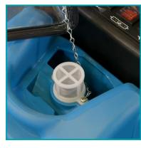
After a few passes, check the waste tank to see that no foam is present. Add extra defoamer if necessary.
