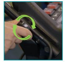
To assemble the machine, screw the two handle knobs into the side of the machine.
