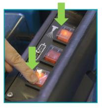
Switch on the accessory spray and vacuum switch button.
