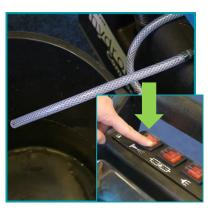
Direct the free end of the hose into a bucket and switch on the accessory spray switch. This will drain any remaining solution.
