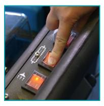
Switch on the vacuum motor and brush drive switches.
