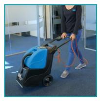
Wheel the machine forward and repeat, slightly overlapping the previous pass. Do not clean any area more than twice, or overwetting could result in carpets shrinking.
