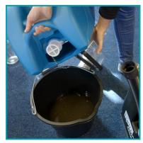
Remove the transparent cover and empty the dirty water. Rinse out the tank with clean water to remove dirt and sediment and replace the tank.
