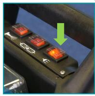
After use and before storage we recommend running the vacuum motor for approximately 2 minutes to allow residual water in the system to be fully sucked into the recovery tank.
