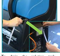
To drain the solution tank, remove the drain hose from the back of the machine, then disconnect the solution hose from the connector and fit the drain hose in its place.
