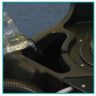
Add approx. ½ litre of clean water to solution tank and drain to flush out the tank and pump.
