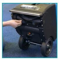
Wipe down the machine, including the underside of the machine. Check the vacuum and brush for any debris.
