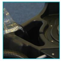
Fill the solution tank with mixed approved and cleaning chemical according to the chemical manufacturer's instructions. Warm water can be used to aid cleaning, however this can increase the risk of colours fading and carpets to shrink. If required, add defoamer solution as per manufacturer's instructions.
