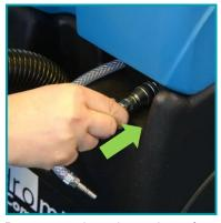
Disconnect the solution hose from the connector on the front of the machine and connect the accessory solution hose to the machine.
