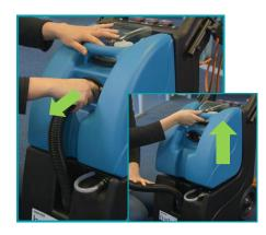
To drain the recovery tank disconnect the vacuum hose and lift off the recovery tank.
