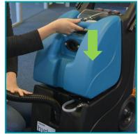
Replace the recovery tank and secure in position.
