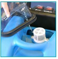
Store machine with recovery tank lid removed. Store the machine in a dry indoor area only.
