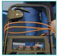
Wrap the supply cord around the handle, ensuring that the plug is not trailing on the floor.
