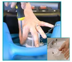
Regularly check the filter by unscrewing the filter, and rinsing out any dirt or debris.
