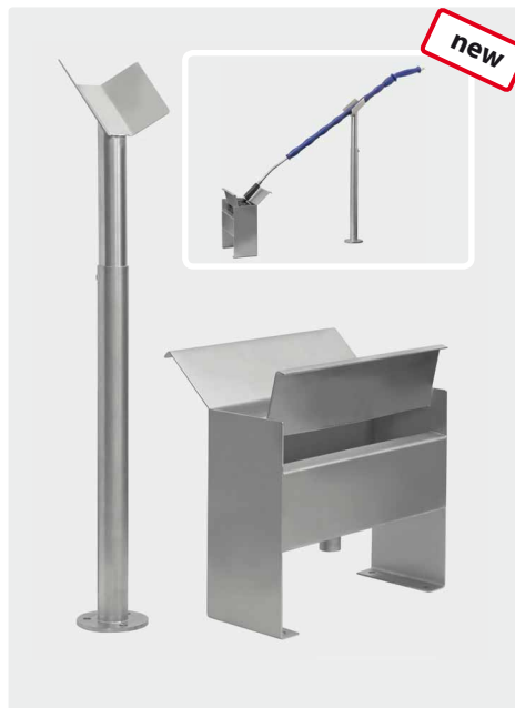
Wash brush holder, two-piece. For floor mounting and positioning for different length of lances. Holder: H x W x D: 315 x 305 x 120 mm. Support pipe: Pipe Ø 42 mm, height adjustable from 570 to 1,000 mm
