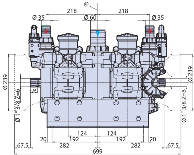
@ = Pump axis - Asse pompa
