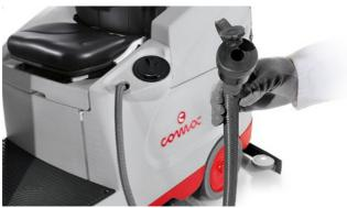
The length of the hose for solution tank filling allows to directly and comfortably reach a water tap. As optional a fast fill system with float is also available to reduce downtimes.
