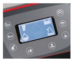
With the versions equipped with CDS dosing system it is possible to be very precise in adjusting water quantity and detergent percentage and to save the settings inside the program selector to use them again automatically for the next cleaning operation.
